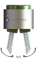
The Flexible Smart Gripper™ (FSG) allows for the picking and placing of a multitude of shapes and sizes due to its patented, FDA compliant silicone fingers, actuated by a fully electric system. The ability to rotate in the Roll degree of freedom, while keeping rigid in the Pitch and the Yaw degrees of freedom, allows for dependable, soft, and flexible gripping of delicate objects.
