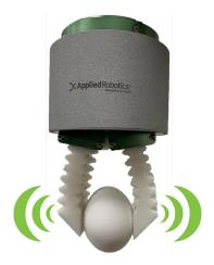
The Enhanced Intelligence version of the FSG provides additional finger positions for grip precision and efficiency, as well as force control, allowing the user to reliably handle delicate objects.
